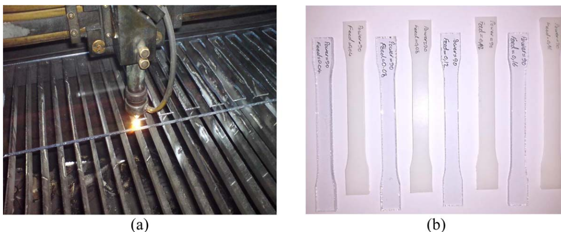
Figure 1. Laser cutting process and produced samples. [Color figure can be viewed in the online issue, which is available at wileyonlinelibrary.com .]
